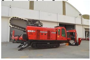
The all new HD 50/100 is a freshly launched rig. It has been designed to be a more compact and cost-effective product. It has a 275 HP cat engine and 200 GPM in-built mud pump, which makes drilling more efficient and having thrust/pullback capacity of 100 tons and high torque. The air-conditioned cabin, with a rotating operator seat, gives a surround view for optimal comfort while monitoring operations. A built-in crane is offered as an option.
