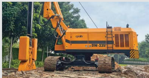
Diaphragm Wall Drilling Rig Apollo DW 235
